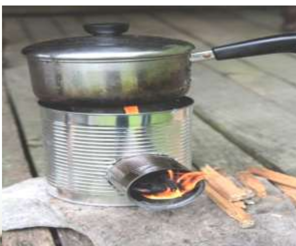
Plate 2: Rocket wood fuel stove
