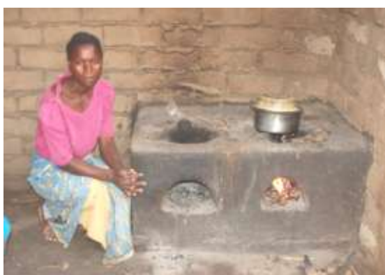
Plate 3: Muddy wood fuel stove
